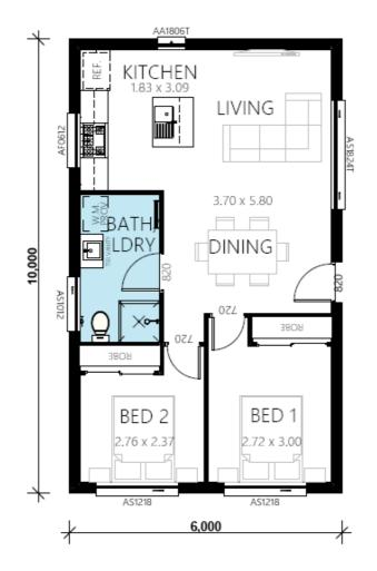
GROUND FLOOR OVERALL WIDTH OVERALL LENGTH 60.00m<sup>2</sup> 6.00m 10.00m
